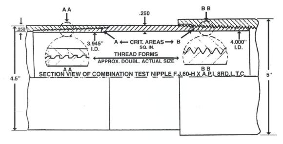
Repeated tests with above setup established two things. the A.P.I. 8rd thread always jumped out at approximately 160,000# tension, leaving the flush joint F.J.60-H undamaged and not tested near to its limit.
