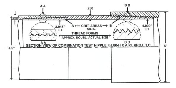
Repeated tests with above setup established two things. the A.P.I. 8rd thread always jumped out at approximately 160,000# tension, leaving the flush joint F.J.60-H undamaged and not tested near to its limit.
